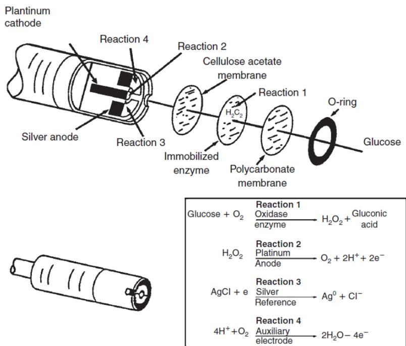
**Figure 2. Schematic of a “first-generation” glucose biosensor.**
