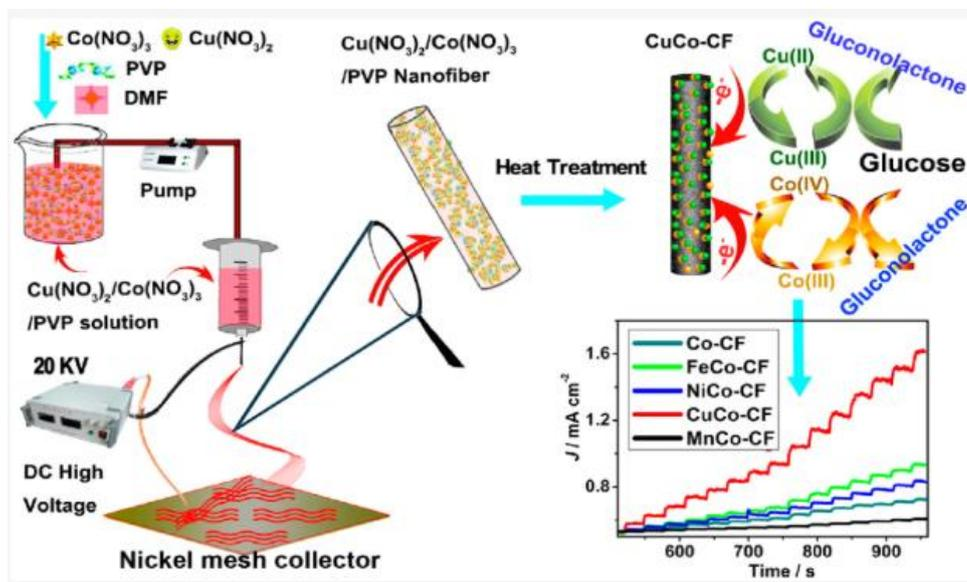
**Figure 4. Biosensor amperometric findings, electrochemical mechanism of electrodes, and processes for synthesising Co/CNFs and MCo/CNFs (where M = Fe, Ni, Cu, and Mn) nanocomposites.**
